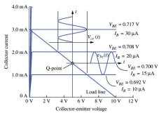
8 mV peak change in  $v_{BE}$  gives 5 mA change in  $i_B$  and 0.5 mA change in  $i_{C}$ .
