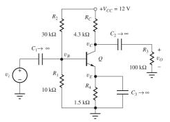
ac coupling through capacitors is used to inject ac input signal and extract output signal without disturbing Q-point
