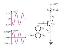
The BJT is biased in the active region by dc voltage source  $V_{BE}$ . e.g., Q-point is set at ( $I_C$ ,  $V_{CE}$ ) = (1.5 mA, 5 V) with  $I_B$  = 15  $\mu$ A ( $\beta_F$  = 100)
