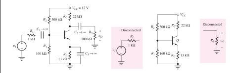
All capacitors in the original amplifier circuit are replaced by open circuits, disconnecting v<sub>I</sub>, R<sub>I</sub>, and R<sub>3</sub> from circuit.
