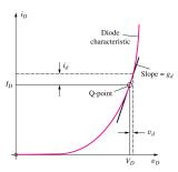
$$g_d = \frac{\partial i_D}{\partial v_D}\Big|_{Q-point} = \frac{I_S}{V_T} \exp\left(\frac{V_D}{V_T}\right) \approx \frac{I_D}{V_T}$$
